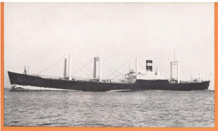
Above: This C-2 vessel is one of a large group—all equipped with G-E geared-turbines—that have established remarkable over-all fuel consumption economies.
