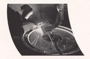
In the low-pressure stages, where the volume of steam is large, diaphragms with cast-in nozzle partitions are used. Annealing and machining complete the diaphragm.
