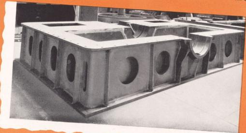
LOWER SECTION of a reduction-gear
